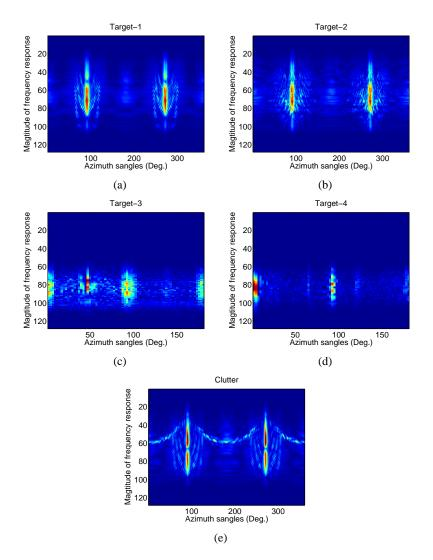
Figure 9: Frequency-domain acoustic responses of the five underwater objects (a) Target-1 (b) Target-2 (c) Target-3 (d) Target-4 (e) Clutter.
