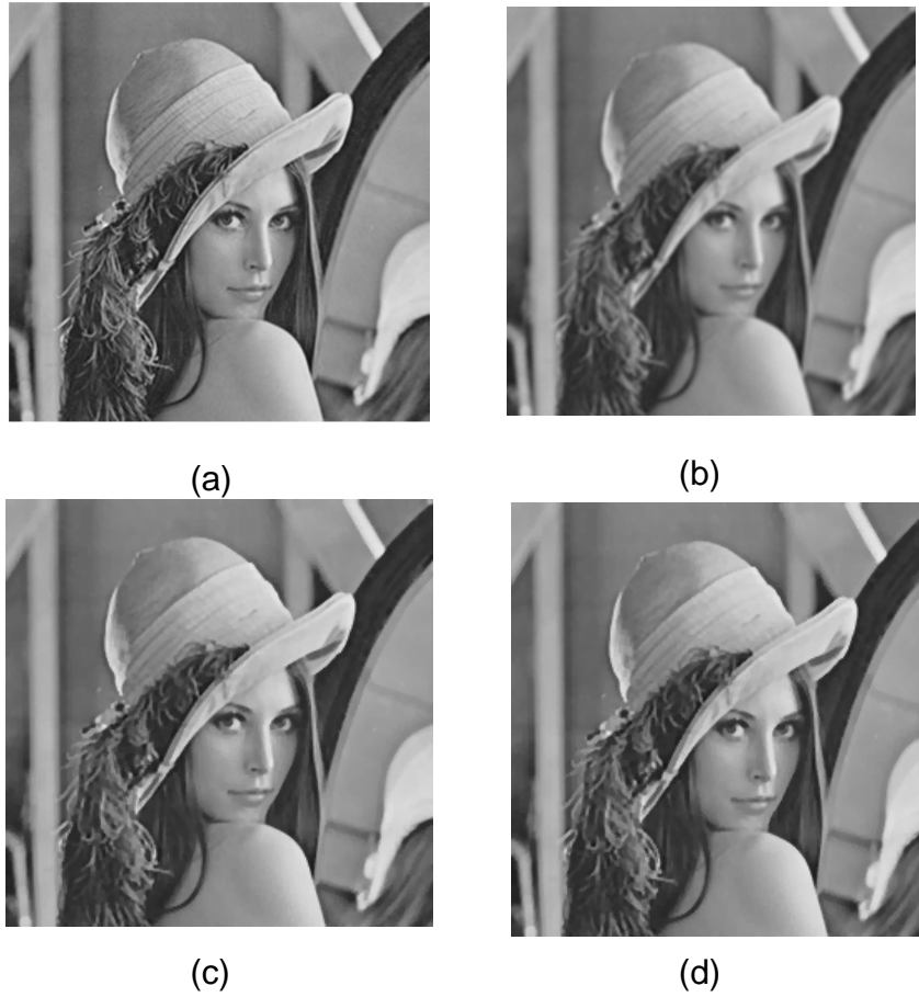
Figure 6: Results of deblurring using fused lasso penalty. Plots (a), (b), (c), and (d) correspond to the original image, the blurred image, the ALIN de-blurred image, and the FISTA de-blurred image, respectively.
