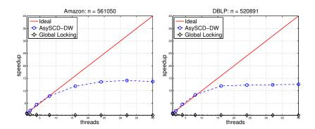
Figure 3: Test problems 3 and 4: Speedup of multicore implementations of DW on up to 40 cores of an Intel Xeon architecture. Ideal (linear) speedup curve is shown for reference, along with poor speedups obtained for a global-locking strategy.
