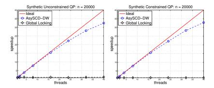
Figure 2: Test problems 1 and 2: Speedup of multicore implementations of DW on up to 40 cores of an Intel Xeon architecture. Ideal (linear) speedup curve is shown for reference, along with poor speedups obtained for a global-locking strategy.
