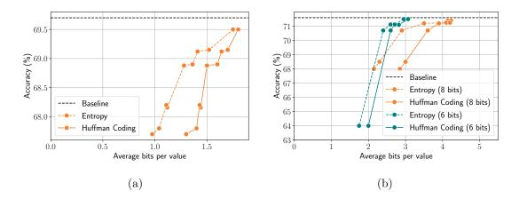
Figure 4: Tradeoff between rate and accuracy for different values of  $\lambda$  (ranged between 0 and 0.3) in (a) ResNet-18 and (b) MobileNetV2 in activations compression. In ResNet-18, the activations are quantized to 5 bits; in MobileNet we show results for activation quantized to 6 and 8 bits.
