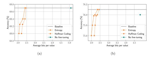
Figure 3: Tradeoff between rate and accuracy for (a) ResNet-18 and (b) ResNet50 in weight compression. The activations are quantized to 8 bits for fair comparison. "No fine-tuning" refers to pre-trained model with activations and weights quantized to 8 bits and the Huffman coding applied to the weights.
