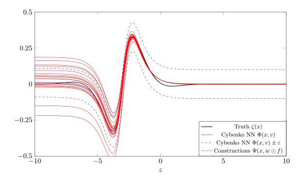
Figure 4: An illustration of function approximation in probability with our construction. Here, M=256, and 20 independent runs of the construction are shown in red. Here,  $\epsilon=0.1$  was chosen for illustrative purposes. Most of the runs lie within  $\epsilon$  distance around the Cybenko neural network from (15), which we approximate with our construction in (16). Altogether, we are approximating the target function  $\zeta$ .
