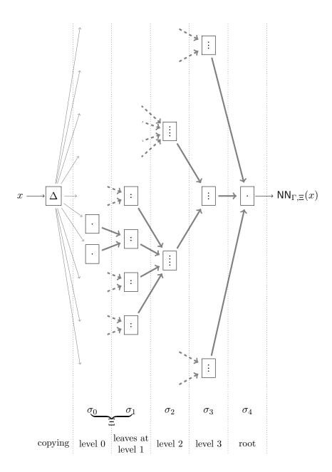
Figure 6: An illustration of how we use the base neural network  $\Psi$  from Figure 5 and a dropout-tree (indicated with thicker arrows) to ultimately construct the larger neural network  $\mathsf{NN}_{\Gamma,\Xi}$  in which edges are being dropped stochastically. Here, L=4.
