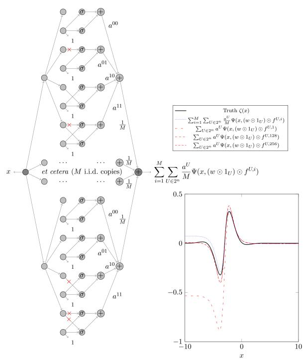
Figure 3: An approximation of  $\zeta$  with a large neural network using dropconnect, based off the base Cybenko neural network in (15) depicted in Figure 1. Adding many independent copies of the network from Figure 2, we are leveraging the law of large numbers as in (16). Different independent copies of the network may have a different realization of the filters, which is here depicted by the red crosses on the edges.
