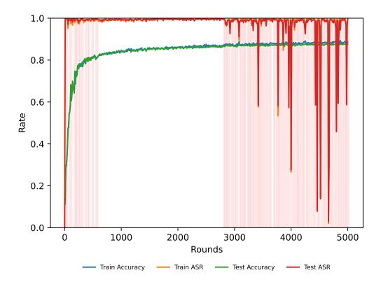
Figure 1: Measurements over the system run time of the 50% Adv. FoolsGold with 10 endpoints total. The red shading indicates periods of time where the attack is toggled "on". We observe that the on-off attack enables the sustenance of an high average attack success rate.
