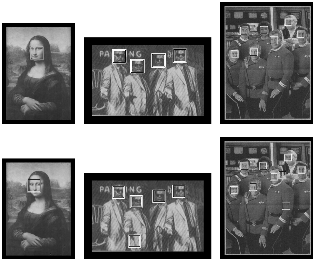
Figure 1: Comparison between a single SVM (top row) dedicated to a nearly fixed pose and our designed network (bottom row) which investigates many poses simultaneously. The sizes of the three images are, left to right, 520 \times 739 , 462 \times 294 and 662 \times 874 pixels. The network achieves approximately the same accuracy as the pose-specific SVM but with order 100-1000 times fewer kernel evaluations. Some statistics comparing efficiency are given in Table 1.
