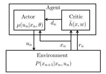
Figure 1: A schematic illustration of the dynamics between the actor, the critic, and the environment. The actor chooses an action,  $u_n$ , according to the parametrized policy  $\mu(u|x,\theta)$ . As a result, the environment proceeds to the next state according to the transition probability  $P(x_{n+1}|x_n, u_n)$  and provides a reward. Using the TD signal, the critic improves its estimation for the environment state values while the actor improves its policy.
