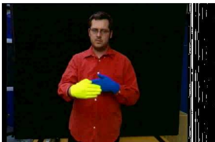
Figure 13: Repetition of the appearance based sub-unit classifier vector. The band down the right hand side of the frame shows the sub-unit level classifier firing patterns for the last 288 frames, the vector for the most recent frame is at the bottom. The previous video during the 288 frames shows four repetitions of the sign ‘Box’.
