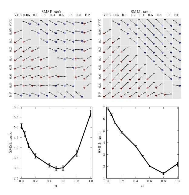
Figure 5: Average ranking of various  $\alpha$  values in the regression experiment, lower is better. Top plots show the pairwise comparisons. Red circles denote rows being better than the corresponding columns, and blue circles mean vice versa. Bottom plots show the ranks of all methods when being compared together. Intermediate  $\alpha$  values (not EP or VFE) are best on average.
