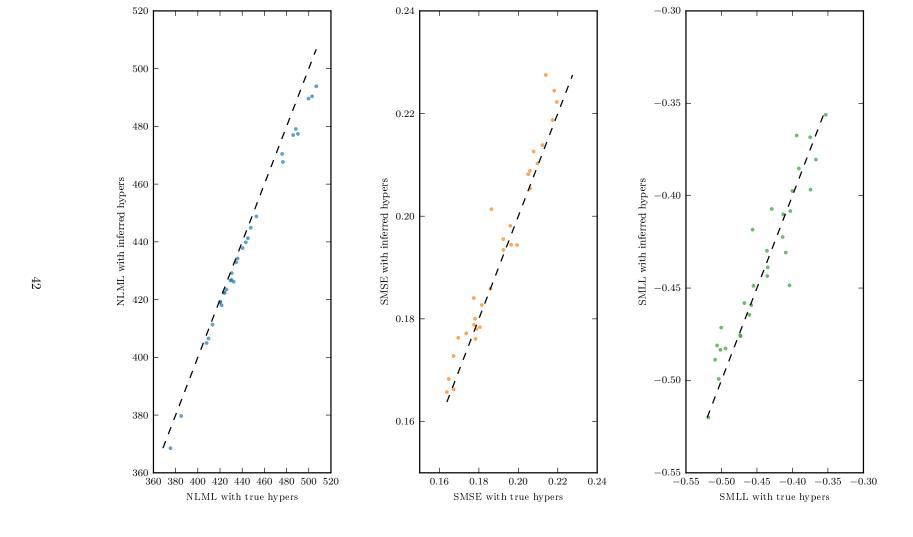
Figure 8: Results on a toy regression problem: Negative log-marginal likelihood, mean squared error and mean log-loss on the test set for full Gaussian process regression on synthetic data sets with *true* hyperparameters and hyperparameters obtained by type-2 ML. Each dot is one trial, i.e. one synthetic data set. The results demonstrate that type-2 maximum likelihood on hyperparameters works well, despite being a little confident on the log-marginal likelihood on the train set.
