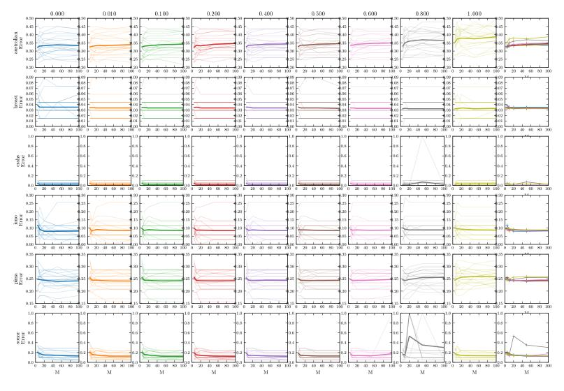
Figure 27: Results on real-world classification problems: Classification error rate on the test set for different data sets, various values of  $\alpha$  and various number of pseudo-points M. Each trace is for one split, bold line is the mean. The rightmost figures show the mean for various  $\alpha$  for comparison. Lower is better.
