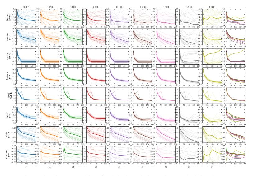
Figure 21: Results on real-world regression problems: Standardised mean log loss on the test set for different data sets, various values of  $\alpha$  and various number of pseudo-points M. Each trace is for one split, bold line is the mean. The rightmost figures show the mean for various  $\alpha$  for comparison. Lower is better.
