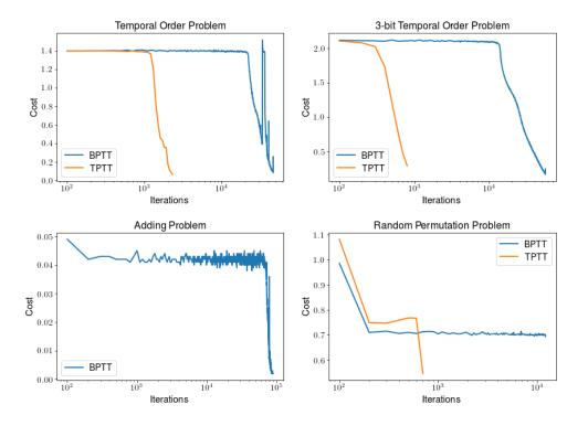
Figure 4: Changes in the training cost for the synthetic problems. The models compared are the ones listed in Table 2. The cost function is averaged over 100 iterations. The iterations are given on a logarithmic scale, as the TPTT network converges significantly faster than the BPTT network.
