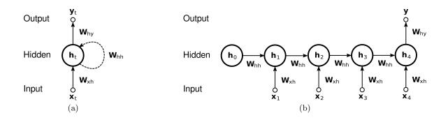
Figure 1: (a) A Simple Recurrent Network with one input unit, one output unit, and one recurrent hidden unit (b) An SRN "unrolled" for four time steps  $(t \in [1, 4])$ . The network computes a single output y, and the initial state  $\mathbf{h}_0$  is initialised with zeros
