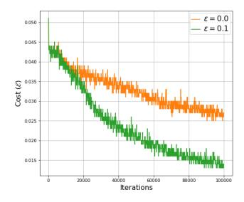
Figure 7: Impact of Gaussian noise on the adding problem with  $t_{max} = 70$ . The learning parameters are set to  $\alpha_i = 0.1$ ,  $\alpha_f = 0.01$ ,  $\alpha_g = 0.01$ , and the network is run with  $\epsilon = 0.0$  and  $\epsilon = 0.1$  for 100,000 iterations. The value of the cost function is averaged over 100 iterations.
