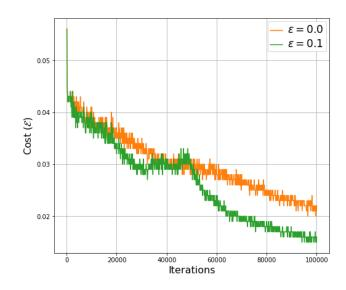
Figure A1: Impact of Gaussian noise on the adding problem with  $t_{max} = 70$ . The learning parameters are set to  $\alpha_i = 0.2$ ,  $\alpha_f = 0.01$ ,  $\alpha_g = 0.05$ , and the network is run with  $\epsilon = 0.0$  and  $\epsilon = 0.1$  for 100,000 iterations. The value of the cost function is averaged over 100 iterations.
