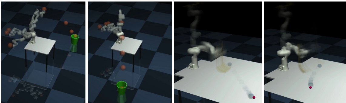
Figure 3: Examples of the performance of policies trained with the GenRL method on the basketball and hockey tasks. For the basketball task, the trained policy can successfully throw the ball into the green basket placed at different random locations, and for the hockey task, the policy can shoot the puck to random target positions illustrated by the red dots.
