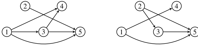
Figure 3: The dependency graphs for the two examples of Figure 2; the left and right graphs correspond respectively to the single- and multi-agent examples presented therein. The active feedback at time t is exactly the set of in-neighbors of the corresponding vertex.
