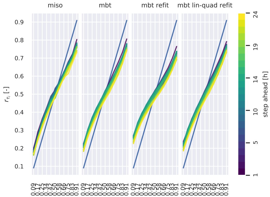
Figure 20: Reliability plots for different models, as a function of \tau_i and the step ahead (line color, from blue to yellow).
