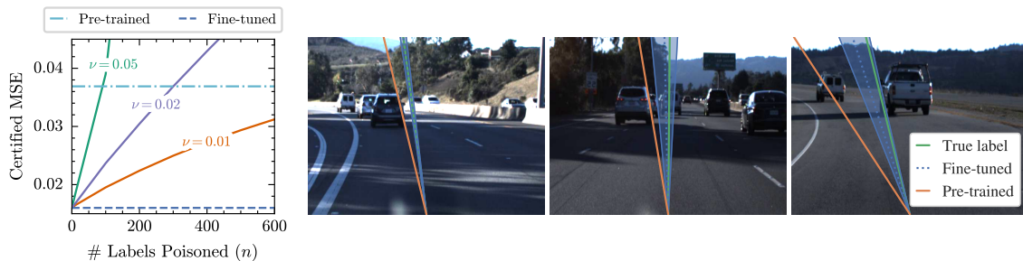
Figure 11: Left: Fine-tuning PilotNet on unseen data with a bounded label-poisoning attack ( q = \infty ). Right: Steering angle prediction before and after fine-tuning ( n = 300, q = \infty, \nu = 0.01 ), indicated by the angle of the lines.
