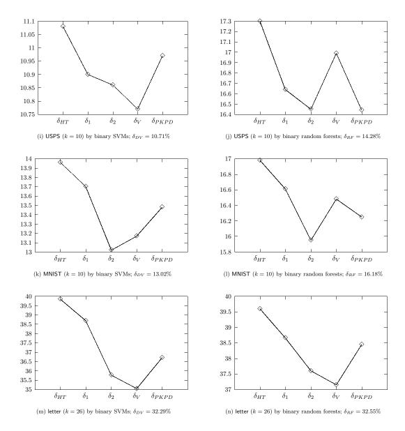
Figure 6: Average of 20 test errors by five probability estimates methods based on binary SVMs (left) and binary random forests (right). Each of the 20 test errors is by 300 training/500 testing points. Caption of each sub-figure shows the averaged error by voting using pairwise SVM decision values ( $\delta_{DV}$ ) and the multi-class random forest ( $\delta_{RF}$ ).
