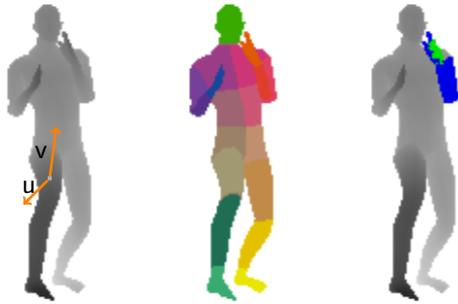
Figure 4. **Left:** Depth image with a candidate feature specified by the offsets  $u$  and  $v$ . **Centre:** Body part labels. **Right:** Left hand joint predictions (green) made by the appropriate class pixels (blue).
