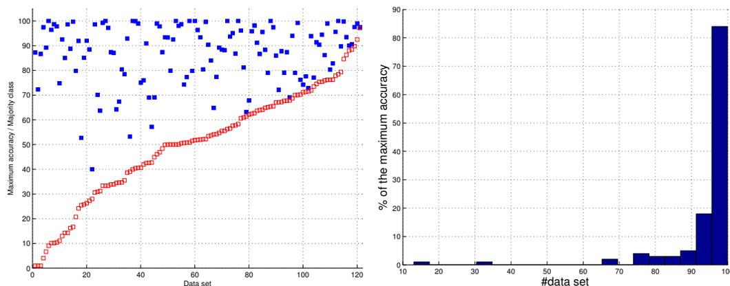
Figure 1: **Left:** Maximum accuracy (blue) and majority class (red), both in % ordered by increasing %Maj. for each data set. **Right:** Histogram of the accuracy achieved by `parRF_t` (measured as percentage of the best accuracy for each data set).
