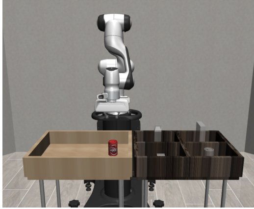
Figure 6: A fetch-and-place robot transfers objects. In dynamic environments, the robot should also be able to handle moving objects within a defined area.
