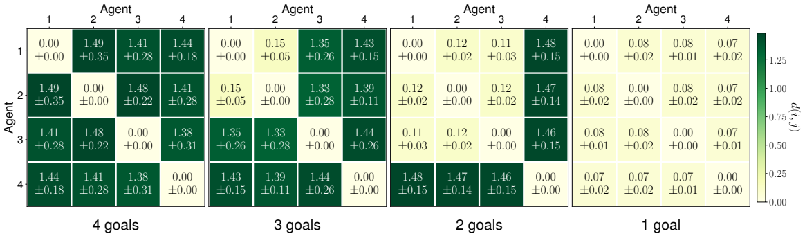
Figure 3: Behavioral distance matrices for the four experiments run on Multi-Agent Goal Navigation . We can observe how, when agents are assigned the same goal, they become behaviorally homogeneous and thus reduce their behavioral distance. We report mean and standard deviation for d(i, j) over 5 random seeds for each experiment. The values are collected after 300 training iterations each performed over 600 episodes of experience.
